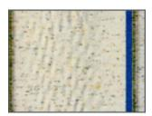
**White Lines or Folds -** Subsequent to handling during fabrication and assembly, acrylic fabrics treated with resins containing fluoride may show small white traces that appear on the fabric due to the stiffness that is caused by the fluoride treatment. These lines are particularly visible in light fabrics as they are held up against the light.
