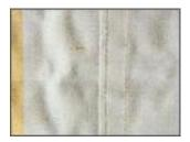
**Stretching of the side hems -** The fabric is usually kept permanently taut using an active spring system. Seams and hems have a reinforcing effect but must also take most strain and withstand high loads. When the fabric is rolled up the hems and seams lay on top of one another, this increases the pressure and tension even more. Seams and hems are pressed flat and increase in length. When the awning is extended out this can lead to the side hems becoming wavy or hanging down.
