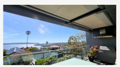
The Albatross Max is made to withstand all weather conditions by using an innovative tension system to secure the fabric on all sides. This eliminates any gaps between the fabric and guide rail, optimising shade coverage and preventing rain from pooling on the awning. For complete all-weather protection, the Albatross Max requires installation at a minimum 15° slope.
